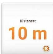
The DistanceToFloor [digit] widget shows the distance to a configurable floor. In order to display the distance, the elevator requires a position sensor, which provides the position values to the display via CANopen lift. In addition, a learning journey must be carried out.
