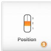
If the display is connected to an absolute position sensor, the widget Position[shaft] can display the current position of the car in the shaft graphically enhanced in a window or in fullscreen mode.
