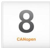
The SimpleFloorIndicator[text] widget displays a floor status sent as text by the controller according to the CANopen Lift standard.
