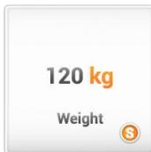
The widget Load[digit] displays the current payload of the lift in kg. To display the measured values, the lift needs to dispose of a load measuring sensor that provides the display the information via CANopen-Lift.
