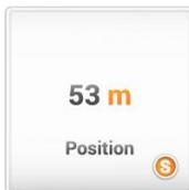
The widget Position[digit] displays the current position of the car in the shaft. The widget can display the absolute height in the shaft as well as the distance to the next floor. To display the measured values the lift necessitates an absolute position sensor that provides the display the values via CANopen-Lift.
