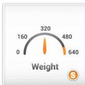
The widget Load[needle] displays the current payload of the lift as a tachometer. The background and the needle, as well as the range from minimum to maximum, are freely configurable. To display the measured values, the lift needs a load measuring sensor that provides the display the information via CANopen-Lift.
