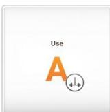
The AssignedLift[text] widget displays the name of the elevator that shall be used. The elevator designation or the text is freely configurable. It requires a CANopen-lift-capable destination call control.
