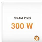
The widget PowerSum[digit] displays the current required energy as a number. To display the measured value, the elevator needs an energy sensor which provides the display with the absolute value via CANopen-Lift.
