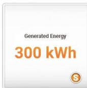
The widget EnergyFedBack[digit] displays the fed energy as a number. To display the measured values, the elevator requires an energy sensor that provides the absolute value to the display via CANopen lift.
